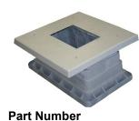
**ENCLOSURE MOUNTING PAD** - The Satellite Assembly shall be provided with an Enclosure Mounting Pad assembly for the purpose of mounting to a "Strong Box" enclosure. This assembly consists of a reinforced plastic support base, a three-sixteenth inch thick 5052 H32 Marine Grade Aluminum mounting pad, and 304-grade stainless steel fastening brackets. The support base shall be installed and compacted in earth allowing the top two inches of the support base to be exposed above the grade.
